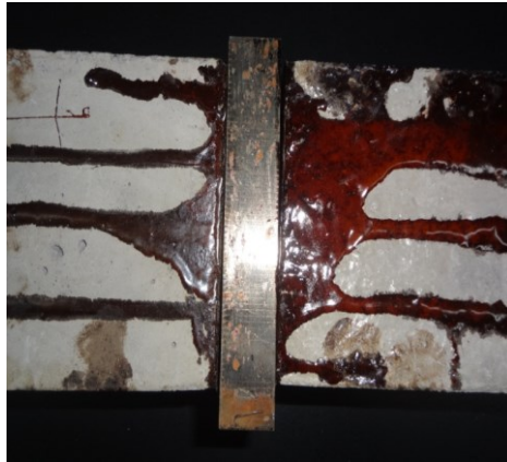
图 10 200℃高温处理后的试件 Fig.10 Test specimen after exposure to 200℃
